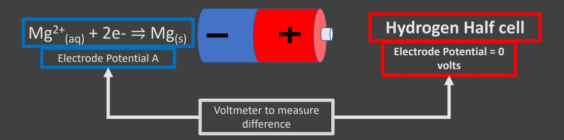
Electrode Potential A = Voltage – Electrode Potential B
