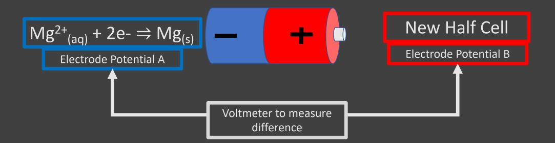
Electrode Potential A = Voltage – Electrode Potential B
