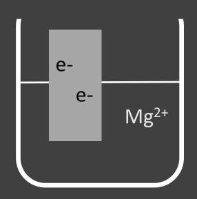
If you place a piece of magnesium metal in water, some of the magnesium atoms will leave their electrons on the metal and into solution as magnesium ions.
