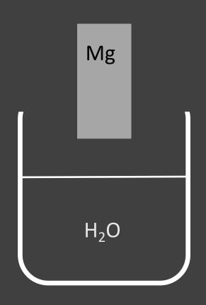
If you place a piece of magnesium metal in water, some of the magnesium atoms will leave their electrons on the metal and into solution as magnesium ions.
