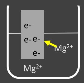
As the negative charge on the magnesium metal increases, magnesium ions are attracted back onto the metal.
